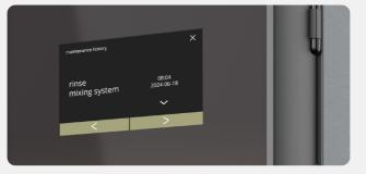
A maintenance history registers when the appliance has been flushed, descaled or when the water filter has been replaced.
